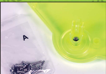
FIGURE 10. Mount the front caster wheel to the base plate. Use the hardware from parts bag A.
